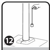
Assemble base cover around the pole with the two nuts and bolts, and then drop the cover over the top of the tilting base.
