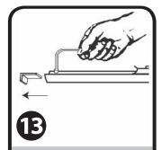
Unscrew both screws at the ends of the aluminum banner crossbar, but do not remove them. Remove the L-Shaped part.
