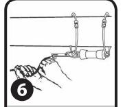
Connect the halyard cable extremity to the counterweight and retaining ring using supplied L-Shaped part.
