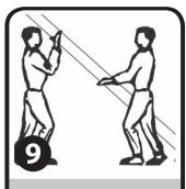
Installer #2 helps lift the pole to vertical position.
