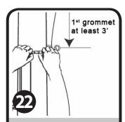
Insert a retaining ring in grommet and secure retaining ring around the pole with a snap hook. Repeat for other grommets.
