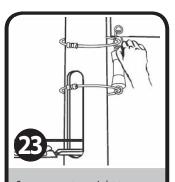
Secure counterweight to banner's bottom grommet using quick link and connect retaining ring. Install last retaining ring on counterweight's bottom eyelet.
