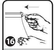
Insert steel L-Shaped part at both ends of crossbar, making sure that the flat metal section is above the banner sleeve.
