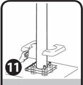
Verify that pole is perfectly vertical and adjust/tighten nuts below the pole plate to achieve verticality.
