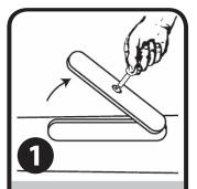
Completely unscrew the access door lock using the supplied special key and remove access door by rotating it 90 degrees.
