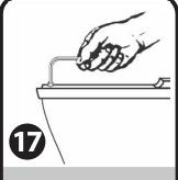
Tighten both screws at the end of the crossbar to secure the banner in the crossbar.
