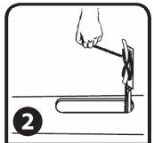
Pull tilting cleat outward and release halyard.
