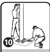
Installer #1 keeps the pole in vertical position while installer #2 secures the tilting base with washers and nuts.
