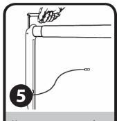
Unscrew screw at end of banner arm so that banner arm can slide with limited pressure over ball bearings.
