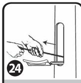
Raise banner. Ensure that crossbar is fully inserted in banner arm. Ensure halyard is tight, then secure it to cleat, push tilting cleat inside pole, and lock cover.
