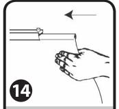
Insert rigid tube in banner sleeve. Slide banner sleeve into crossbar, making sure the grommets are on pole side.
