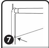
Verify that halyard cable is properly positioned in the pulley which is located in the middle of the banner arm.
